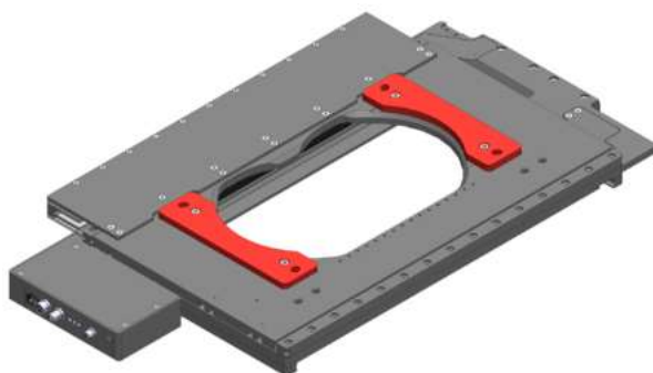
1a. Two piece adaptor plates: Flip the stage upside down. Secure each mounting adaptor to the stage using 2 M4 x 08mm socket cap screws.
